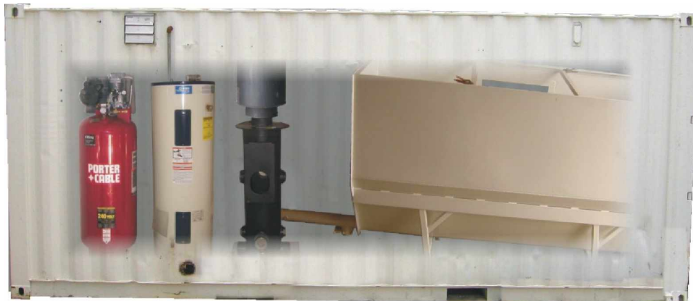
A 20' shipping container with a look inside to the Biomass Furnace's air compressor, water tank, gasifier and hopper
