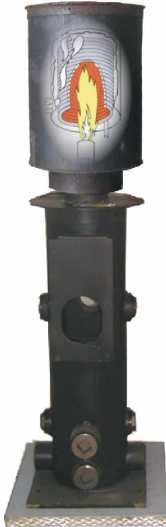
The gasifier and flash boiler
